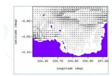
Figure 10. Current Pattern in Highest Tide with Maximum Velocity 0.69 m/s
